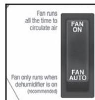
Turning the fan switch “FAN ON” will cause the unit’s internal blower to run continuously, whether the unit is dehumidifying or not. This function is desirable if the unit is used for air circulation or filtration. Turning the fan switch to “FAN AUTO” will cause the unit’s internal blower to run only while the unit is dehumidifying.
